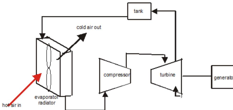
A Cold Engine is a refrigeration system, (heat pump) with a turbine added.
